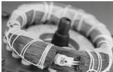
Fig. 46 Thermal switch incorporated in windings
