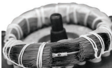
Fig. 44 PTC sensor incorporated in windings
